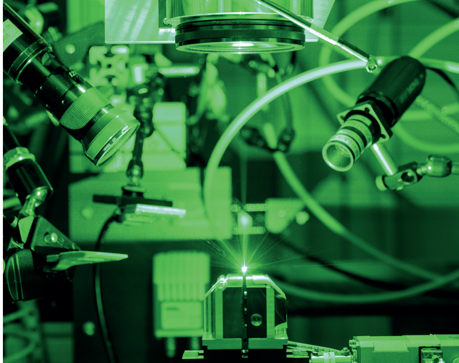
1 Analysis of steam capillaries from synchrotron data, © TRUMPF. 2 Laser-beam welding with green laser, © TRUMPF.
